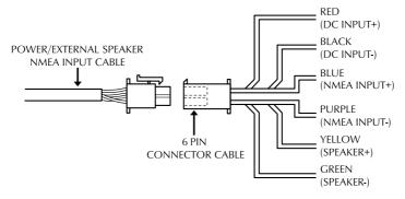
Figure 2-3 Power/External Speaker/NMEA Cable and 6 Pin Connector
